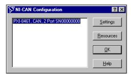
**Figure 2-3.** PXI-8461 That Is Working Properly
